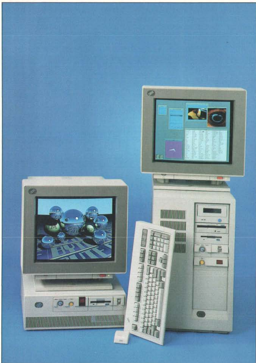
IBM's POWERstation 320 desktop and POWERstation 530 deskside systems. The desktop unit (left) is showing a ray tracing generated by the high-performance three-dimensional graphics board. The deskside system (right) is running OSF/Motif.
